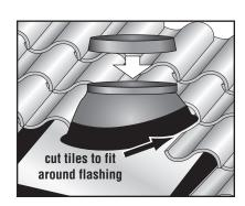
step 6 At the high side of the roof towards the ridge, replace the tiles over the skirt. Cut tiles to fit around flashing. Some furring strips may need to be replaced on top of flashing footprint to support tiles. Replace the tiles on the low side
