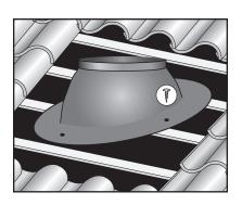
**STEP 4** Install the flashing skirt over the flashing and press down the rubber ring all around the installed flashing.
