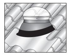
of the roof, but keep skirt above the tiles and reshape the skirt aluminum to form around the tiles.
