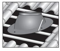
will be installed and mark around the flashing footprint onto the furring strips. Remove the portion of the furring strips where the flashing will be installed (allowing the flashing to sit directly on roof sheathing).
