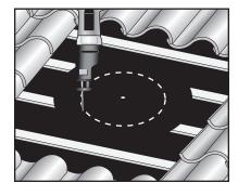
than the area marked in previous step. **NOTE**: A larger hole can be cut to accommodate angled pipe installations.
